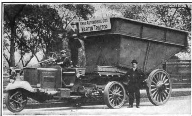
Martin tractor manufactured by Knox Automobile Company, Springfield, Mass., attached to a 15-ton capacity ash wagon, the combination being 12 feet high and 26 feet long
